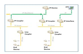
All KNX telegrams between the two (or more) IP Couplers are encrypted
