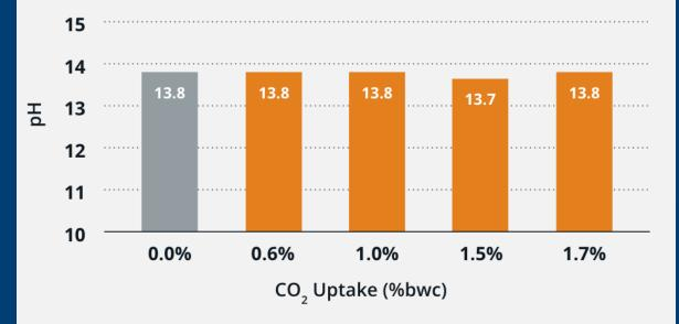
Testing has shown that early carbonation has no impact on the pH of concrete, and therefore has **no impact on corrosion.**
