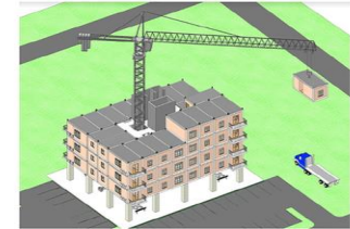
(e) Module lifting and installation at site
