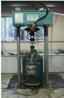
Large-scale triaxial apparatus
